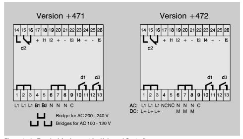
Figure 1 - 3. Terminal Assignment for Universal Controller
