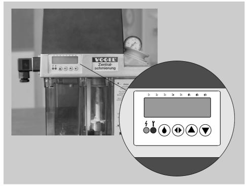
Figure 1 - 2. Operating Display of VOGEL Universal Controller for Industrial Lubrication System, Version I, Installed in Compact System
