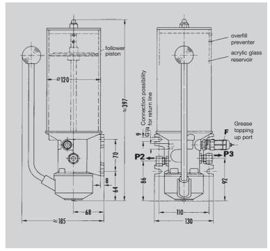
Use connection fittings with cutting-sleeve screw unions to DIN 2353.
